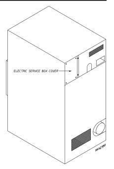
Providing local codes permit, power to a gas dryer can be made by the use of a flexible U.L. listed power cord or pigtail (wire size **must conform** to rating of dryer), or the dryer can be hard wired directly to the service breaker panel. In <u>ALL</u> cases, a strain relief **must be** installed where the wiring enters the dryer and service box area.
